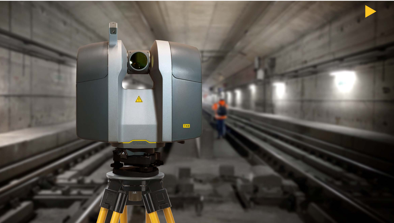
The Trimble TX8 3D Laser Scanner delivers 7-mm accuracy in a railway tunnel survey.
