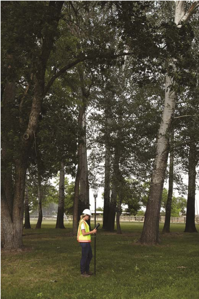
Figure 2: Trimble R10 receiver with Trimble 360 technology under tree canopy
